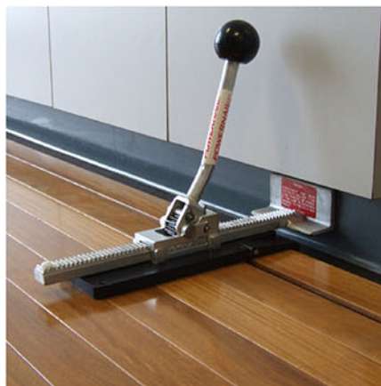
Use under a toe-kick to tighten and hold boards in place.
